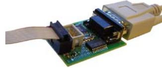
**Figure 3-4.** AVRISP with 6-pin ISP Connector
