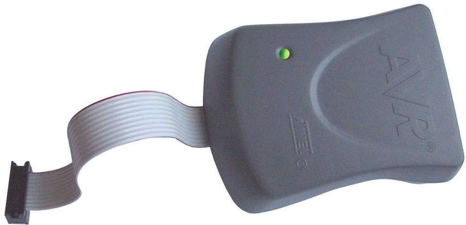
The AVR<sup>®</sup> In-System Programmer (AVRISP) from Atmel<sup>®</sup> is a professional low-cost In-System Programmer covering all AVR 8-bit RISC Microcontrollers. The programmer connects to a PC through a standard RS-232 serial interface and draws the necessary power from the target board eliminating the need for an additional power supply.
