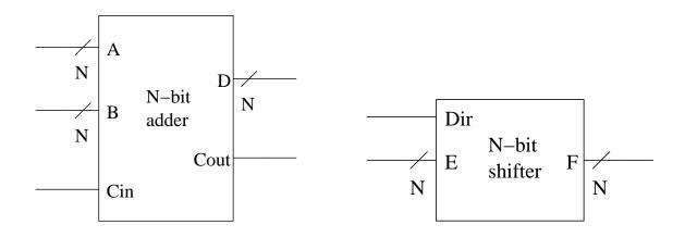
The N-bit adder takes three inputs A, B, and  $C_{in}$ , and produces two outputs D and  $C_{out}$ .
