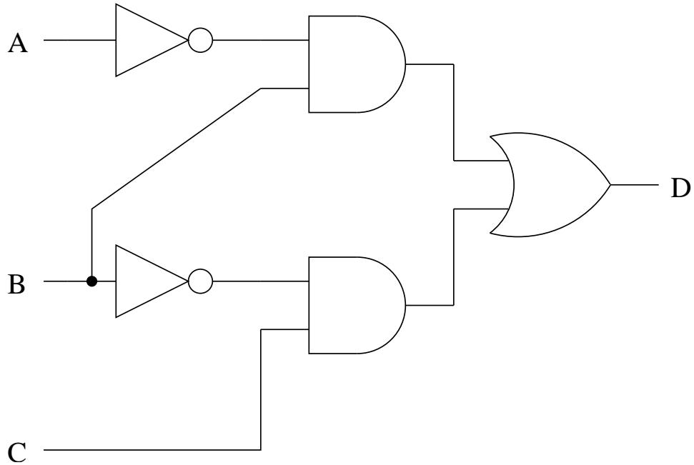
1. Redesign this circuit such that it implements the same function, but uses only NAND and NOT gates. Show this new circuit.
