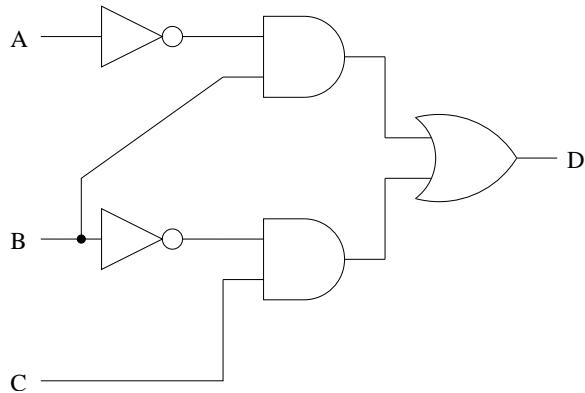
1. (10pts) Redesign this circuit such that it implements the same function, but uses only NAND and NOT gates. Show this new circuit.
