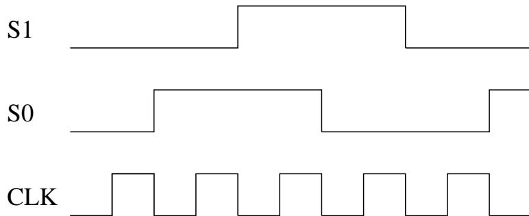
2. Assume  $D = 0$  and an initial condition of  $S1 = 1$  and  $S0 = 0$ . Show the timing diagram for 5 complete clock cycles.
