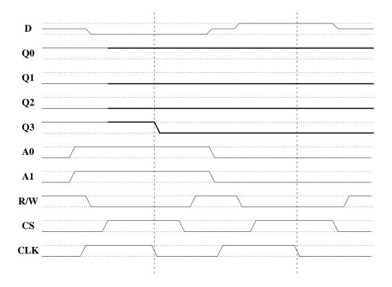
Both memory operations are write operations (to elements 3 and 0, respectively). Note, however, that the state of Q0 does not change (it was already in a state of "1").
