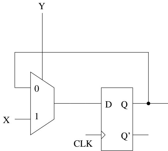
(15pts) Explain in detail what this circuit does in terms of its inputs ( $X$ ,  $Y$ , and  $CLK$ ). (Multiplexer notation note: the 0 and 1 tell you which input is selected when  $Y$  is in these states)
