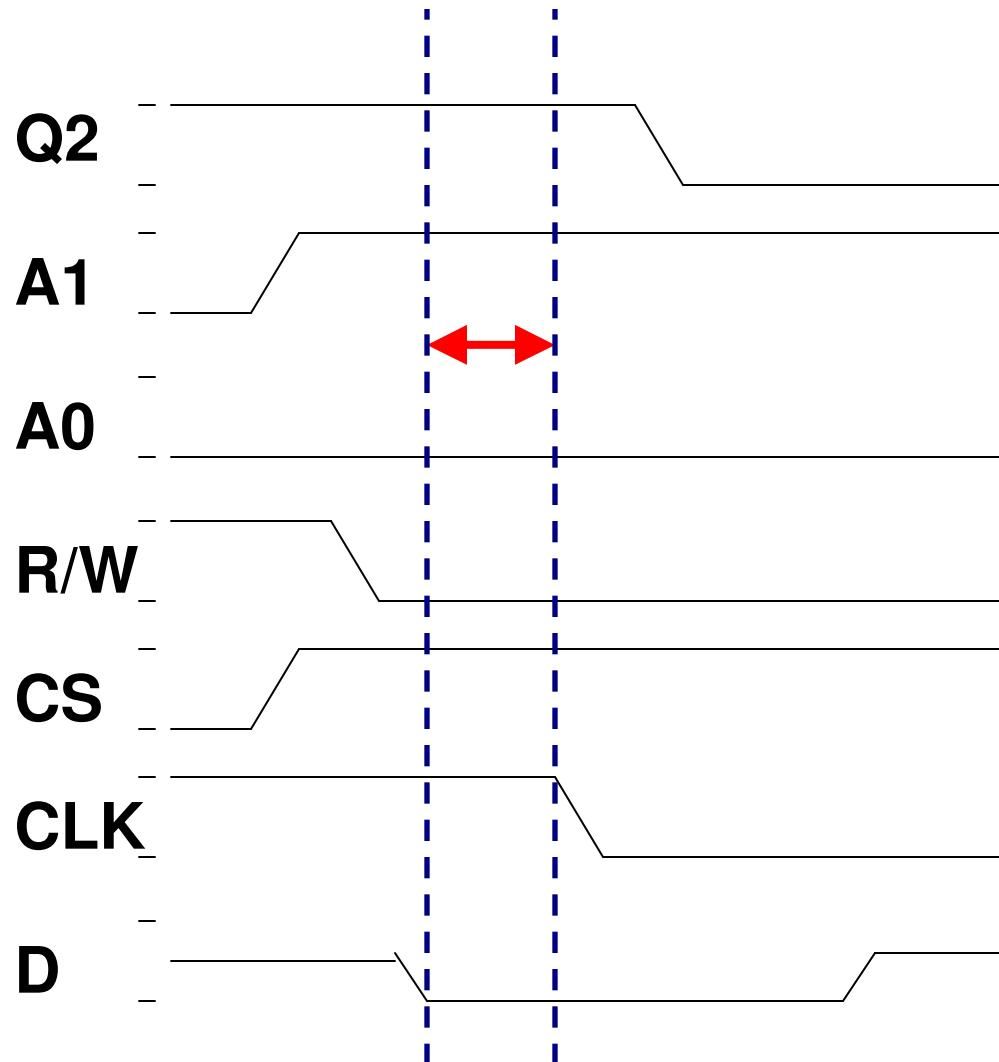
**Setup time:** all inputs must be valid during this time
