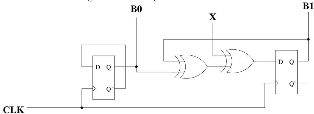
1. (10pts) Assume that the initial state is:  $B0 = 0$  and  $B1 = 0$ . Assume also that  $X = 0$ . Show the timing diagram for  $B0$  and  $B1$  as the clock ( $CLK$ ) is pulsed.
