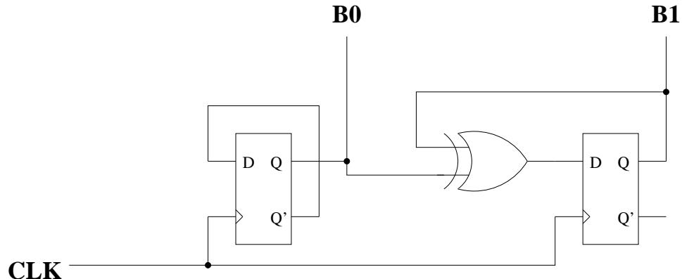
1. (10pts) Assume that the initial state is:  $B0 = 0$  and  $B1 = 0$ . Show the timing diagram for  $B0$  and  $B1$  as the clock ( $CLK$ ) is pulsed.
