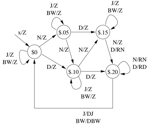
Alter this vending machine such that if three nickels are inserted (starting from state \$0), then a dime is returned immediately and the vending machine still maintains a state of \$.15.
