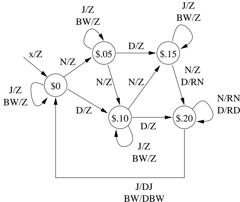
Alter this vending machine such that if three nickels are inserted (starting from state \$0), then a dime is returned immediately and the vending machine
