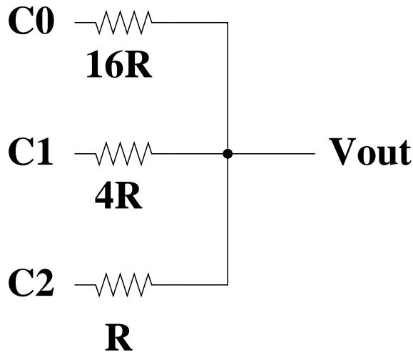
(20pts) Show  $V_{out}$  as a function of  $C_0$ ,  $C_1$ , and  $C_2$ . Show your derivation.
