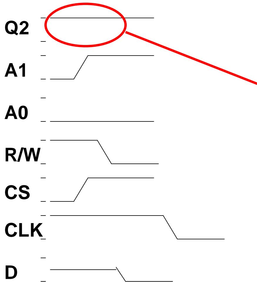
Memory element 2 is initially in a high state
