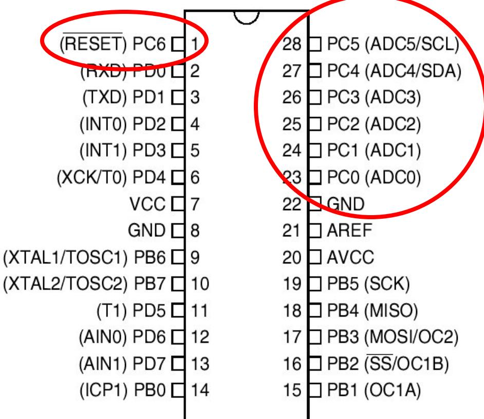
The diagram shows the pinout for an Atmel Mega8 microcontroller in a PDIP package. The pins are numbered 1 through 28. The pins are arranged in two columns. The left column contains pins 1 through 14, and the right column contains pins 15 through 28. The pins are labeled with their functions. Two pins are highlighted with red circles: pin 1 is labeled  $\overline{\text{RESET}}$  and PC6, and pin 28 is labeled PC5 (ADC5/SCL). The functions for the other pins are as follows:
