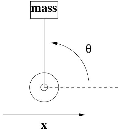
A *bang-bang* controller produces motor commands (in this case, velocity motor commands) depending on the orientation of the pendulum:
