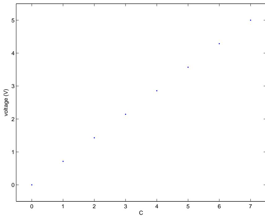
*Note: this is a 3-bit digital to analog converter.*
