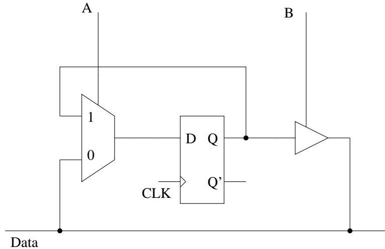
1. (10pts) Suppose that  $Q$  is initially set to 1. If  $A = 1$ ,  $B = 0$ ,  $Data = 0$  and the clock transitions from high to low, what happens to  $Q$  and when?
