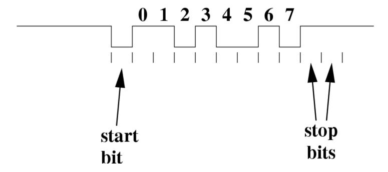
The stop bits allow the receiver to immediately check whether this is a valid frame
