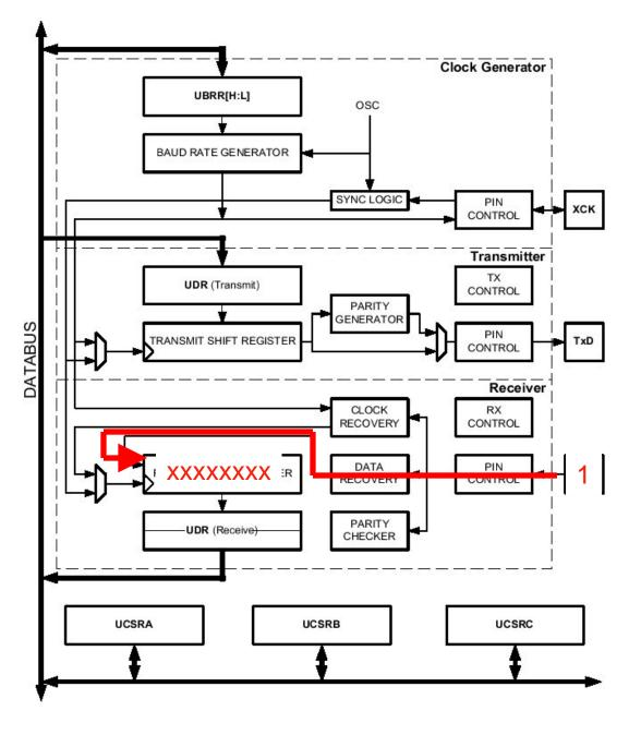
"1" is shifted into the most significant bit (msb) of the shift register
