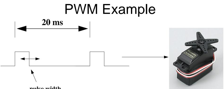
pulse width determines motor position
