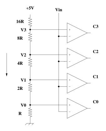
Assume that R is known and that the analog comparators are powered with +5V.
