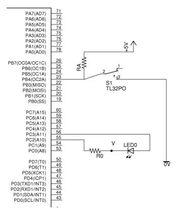
Assume that DDRC = 0xC,  $V_f = 3V$  and  $R0 = 100\Omega$ .
