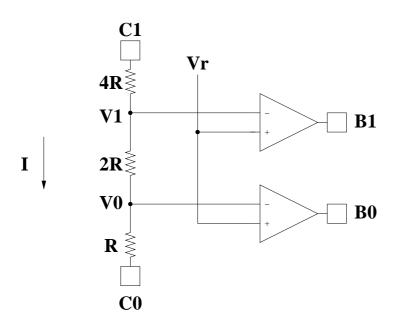
$C_1$  and  $C_0$  are logical values determined by your Atmel Mega processor (i.e., 0 and 1). The voltage at pin i is  $5C_i$ .  $B_1$  and  $B_0$  are inputs into the processor. Assume that the analog comparators produce an output of 0V or 5V.
