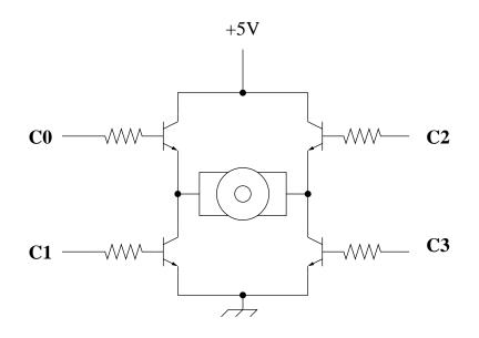
14. (5 points) What configuration of C signals would result in a dynamic braking of the motor?
