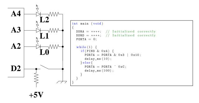
17. (5 points) What is the correct initialization for DDRD given the circuit? A. 0xFF B. 0x38 C. 0x3C D. 0x1C E. Answer not shown
