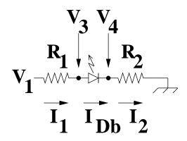
Assume  $R_1 = 100\Omega$ ,  $R_2 = 300\Omega$  and  $V_{fb} = 2V$ .
