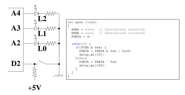
17. (5 points) What is the correct initialization for DDRD given the circuit?
