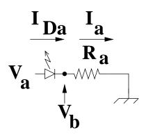
Assume  $R_a = 500\Omega$  and  $V_{fa} = 3V$ .
