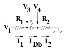
Assume  $R_1 = 100\Omega$ ,  $R_2 = 300\Omega$  and  $V_{fb} = 2V$ .
