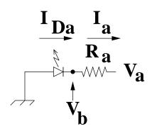
Assume  $R_a = 200\Omega$  and  $V_{fa} = 1V$ .
