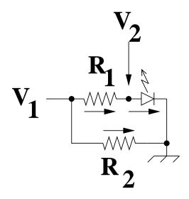
Assume  $R_1 = 100\Omega, R_2 = 1000\Omega$  and  $V_f = 3V$ .
