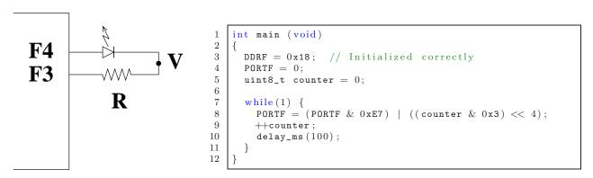
Assume  $R = 400\Omega$ ,  $V_f = 1V$  and the maximum voltage output from a microprocessor pin is 5V.
