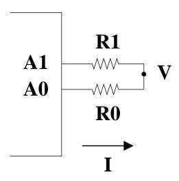
Assume  $R_0 = 500\Omega$ ,  $R_1 = 1000\Omega$  and the maximum voltage output from a microprocessor pin is 5V.
