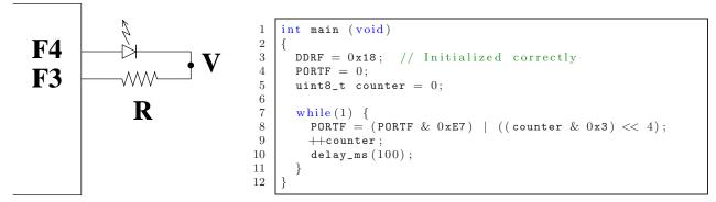
Assume  $R = 400\Omega$ ,  $V_f = 1V$  and the maximum voltage output from a microprocessor pin is 5V.
