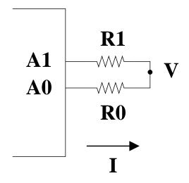
Assume  $R_0 = 500\Omega$ ,  $R_1 = 1000\Omega$  and the maximum voltage output from a microprocessor pin is 5V.
