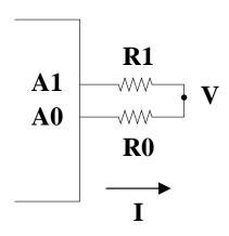
Assume  $R_0 = 1500\Omega$ ,  $R_1 = 500\Omega$  and the maximum voltage output by a microprocessor pin is 5V.
