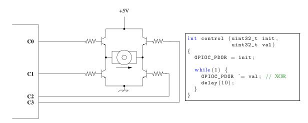
Assume that Port C, pins 0..3 are configured as digital output pins. Also assume that the motor can be modeled as a  $1\Omega$  resistor.
