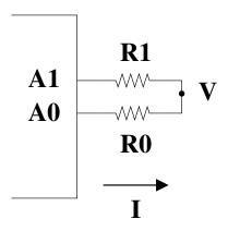
Assume  $R_0 = 1500\Omega$ ,  $R_1 = 500\Omega$  and the maximum voltage output by a microprocessor pin is 5V.
