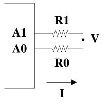
Assume  $R_0 = 1500\Omega$ ,  $R_1 = 500\Omega$  and the maximum voltage output by a microprocessor pin is 5V.
