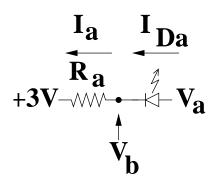
Assume  $R_a = 1000\Omega$  and  $V_{fa} = 2V$ .
