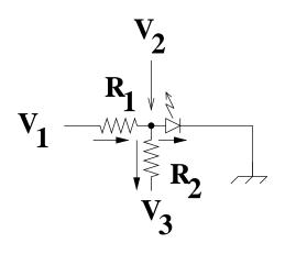
Assume  $R_1 = 100 \Omega$ ,  $R_2 = 300 \Omega$  and  $V_f = 1 V$ .
