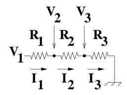
Assume  $R_1 = 100 \ \Omega, \ R_2 = 200 \ \Omega, \ R_3 = 300 \ \Omega.$
