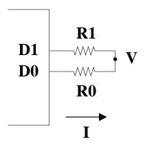
Assume  $R_0 = 50\Omega$ ,  $R_1 = 150\Omega$  and the maximum voltage output by a microprocessor pin is 5V. Also assume that D0/D1 have been configured as output pins.
