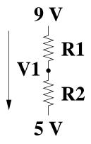
11. (8 points) Assume that  $R_1 = 300\Omega$  and  $R_2 = 100\Omega$ . What is  $V_1$ ?
