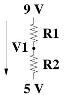
13. (8 points) Assume that  $R_1 = 300\Omega$  and  $R_2 = 100\Omega$ . What is  $V_1$ ? A. 1 V B. 3 V C. 6 V D. 8 V E. Answer not shown
