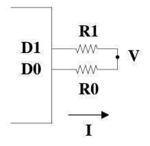
Assume  $R_0 = 50\Omega$ ,  $R_1 = 150\Omega$  and the maximum voltage output by a microprocessor pin is 5V. Also assume that D0/D1 have been configured as output pins.
