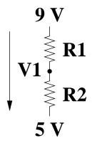
13. (8 points) Assume that  $R_1 = 300\Omega$  and  $R_2 = 100\Omega$ . What is  $V_1$ ? A. 1 V B. 3 V C. 6 V D. 8 V E. Answer not shown
