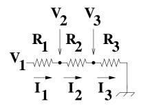
Assume  $R_1 = 200 \Omega$ ,  $R_2 = 100 \Omega$ ,  $R_3 = 200 \Omega$ .
