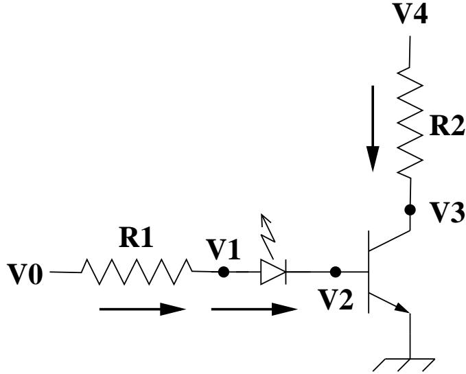
Assume  $V_{fD} = 1V$ ,  $V_{fT} = 0.5V$ ,  $g = 100$ ,  $R1 = 1K\Omega$ ,  $R2 = 100\Omega$  and  $V4 = 10V$ .
