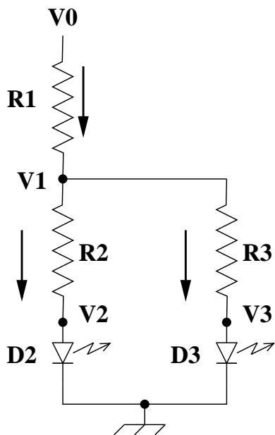
Assume  $R2 = R3 = 0$ ,  $R1 = 500\Omega$ ,  $V_{fD2} = 1V$  and  $V_{fD3} = 2V$ .
