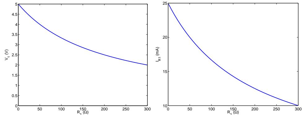
2. (10pts) Assume  $R_2 = 300 - R_1$ . Show  $V_1$  and  $I$  as a function of  $R_1$  (same range). Show your derivation.
