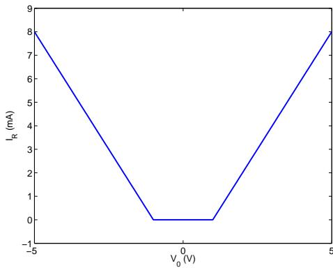
The key is: no matter what  $V_0$  is, current through the resistor is never negative. This is what we refer to as a *rectifier*.
