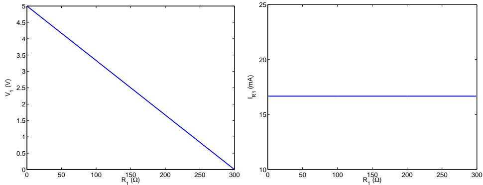
This second case is a type of variable resistor that we refer to as a *linear potentiometer*. These devices have 3 pins: at  $V_0$ ,  $V_1$  and ground in our circuit. The resistance from  $V_0$  to ground is constant (i.e., the sum of  $R_1$  and  $R_2$  remains constant). However, the voltage at the midpoint will vary through the range of  $V_0$  to ground, depending on how the “wiper” is set.
