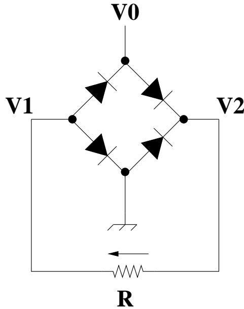
2. (20pts) Consider the above circuit. Assume  $V_f = 0.5V$  and  $R = 500\Omega$ . Show  $IR$  as a function of  $V_0$ . Show your derivation.
