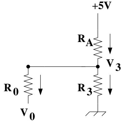
Where  $R_A = R_5 + \frac{R_1 R_2}{R_1 + R_2}$ .
