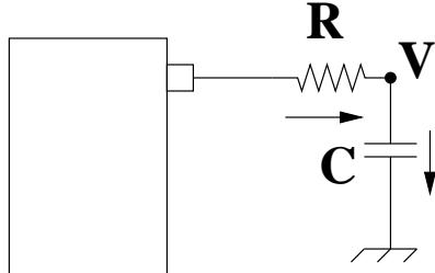
Assume that a PWM cycle starts at time  $t = 0$  with the pin in a state of  $5V$ . At time  $t_1$ , the pin state changes to  $0V$ . At time  $t_2$ , the PWM cycle ends (and the new cycle begins).
